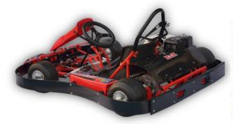
Roll Hoop, Seatbelt and Axle cover ensure complete safety to the driver
