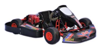
It is driven by a reliable and high revving Honda GX35 OHC engine.
