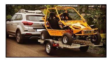
railers are also available to transport the Sidewinder, it can be used to haul a kart or a buggy or motorbikes. It hitches onto most cars and features all the possible safety required for the application, including brakes, taillights, traffic indicator, hazard lights, handbrake, rear stops to prevent roll off, leaf springs with hydraulic damper suspension, easy loading and unloading, etc.
