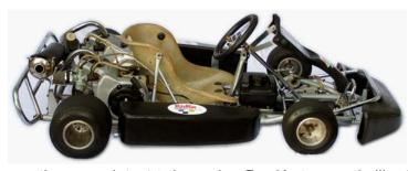
powered by TWIN Briggs & Stratton Vanguard 6 hp engines will be provided by VCR Motor Sport (a sister concern).
