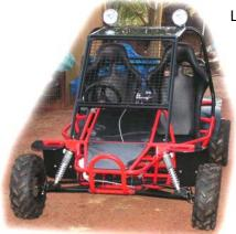
Long travel adjustable fully independent suspension lets the Pathfinder take on most types of terrain with relative ease. With a ground clearance of over 10 inches, the Pathfinder
