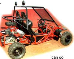
almost anywhere. The exhaust and engine air intake are mounted up and away from the ground so traversing shallow streams and rivulets is not an impediment.
